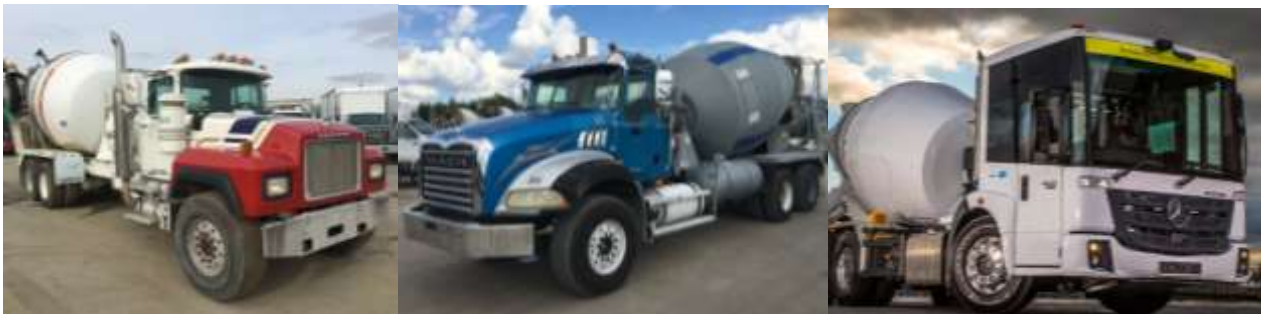
Left: 1970s cement truck. Middle: Typical late 2010s low-visibility truck, soon to be banned in London UK. Right: Modern truck with high-visibility cabin, camera sensor systems, & side guards.
